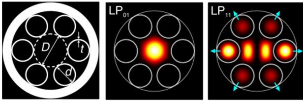
**Fig. 11.** (a) Sketch of the structure, with the key dimensions marked in core diameter  $D$ , capillary inner diameter  $d$ , and wall thickness  $t$ . (b) Fundamental  $LP_{01}$  mode is strongly confined. (c) HOMs experience high loss because they are coupled to modes in the capillaries. Light in the core leaks out to the solid glass sheath (indicated by blue arrows). Reprinted with permission from [42]. Copyright 2016 Optical Society of America.
