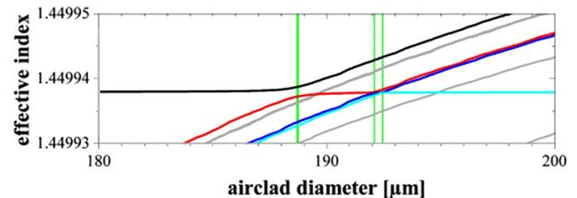
**Fig. 9.** Detailed plot of one broad and two narrow avoided crossings (marked in green vertical lines). The modes involved in avoided crossings are shown in black, red, green, and blue. Reprinted with permission from [29]. Copyright 2011 Optical Society of America.
