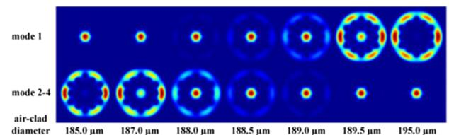
**Fig. 10.** Transverse mode profiles of the modes involved in the broad avoided crossing in Fig. 9 around an air-clad diameter of  $188.5 \mu\text{m}$ . Across the avoided crossing, the former fundamental mode evolves into an HOM, and an HOM takes over the role as the fundamental mode. Reprinted with permission from [29]. Copyright 2011 Optical Society of America.
