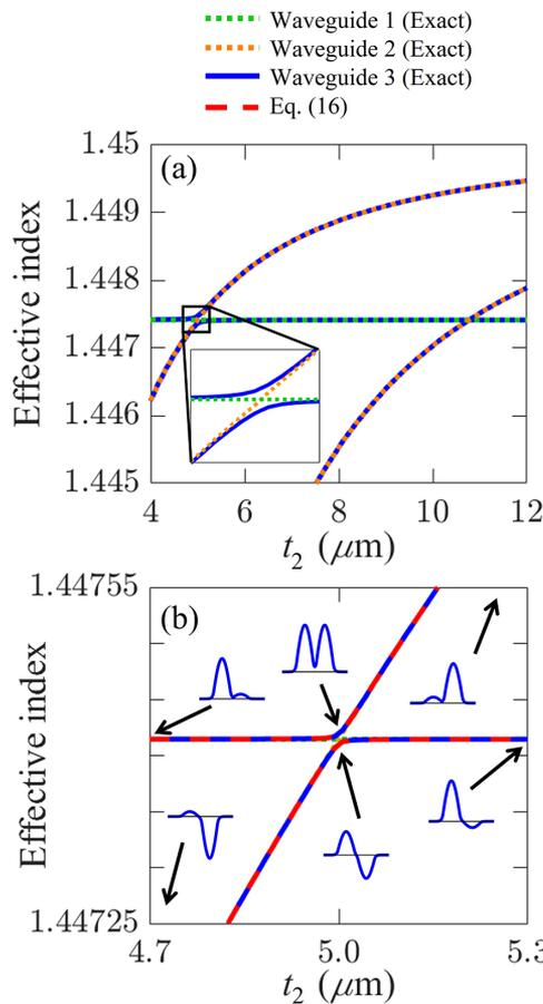
**Fig. 2.** (a) Effective index for the fundamental core mode in waveguides 1 and 2 (dashed curves) and waveguide 3 (solid curve) as a function of  $t_2$ . Inset in (a) shows a magnified plot so that the avoided crossing may be easily seen. (b) Magnified plot in (a) around the first avoided crossing at  $t_2 = 5 \mu\text{m}$ . Insets show mode profiles in waveguide 3. The red dashed curve shows the effective index obtained from Eq. (16).
