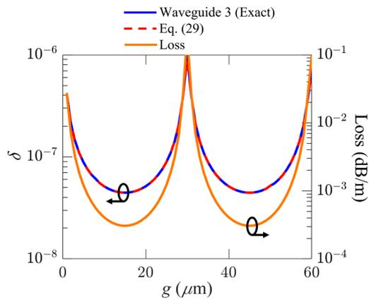
**Fig. 7.** Width of the avoided crossing and loss during an avoided crossing as a function of the width of air gap  $g$  with  $t = 0.72 \mu\text{m}$  and  $W_{\text{core1}} = W_{\text{core2}} = 30 \mu\text{m}$ .
