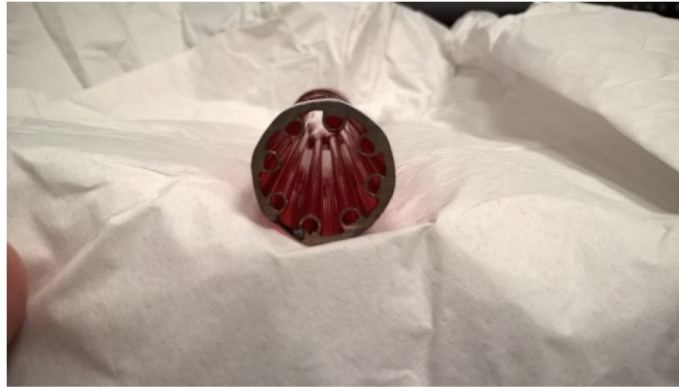
Fig. 1. Diamond saw cut extruded preform.
