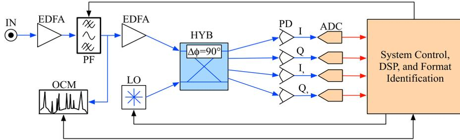
Fig. 1. Format identification system block diagram. IN—optical input, EDFA—erbium doped fiber amplifier, PF—programmable optical filter, OCM—optical channel monitor, LO—local oscillator, HYB— $90^\circ$  optical hybrid, PD—photodiodes, ADC—analog to digital converters, DSP—digital signal processing.
