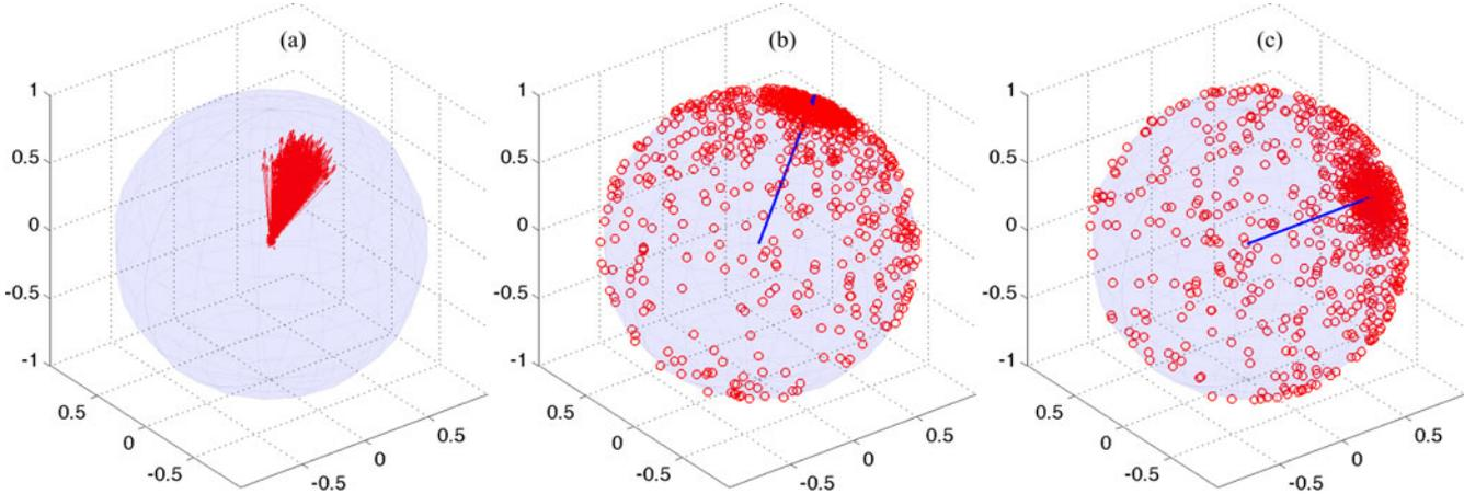
Fig. 3. Stokes vectors of symbol-centered data are shown as red arrows in (a). In (b) and (c) normalized Stokes vectors of symbol-centered data are shown as red circles on the surface of a unit sphere. The normalized vector sum of the Stokes vectors (average SOP) is represented as a blue arrow. The blue arrow indicates the received average SOP before (b) and after (c) rotating the SOP to lie along the  $x$ -axis.
